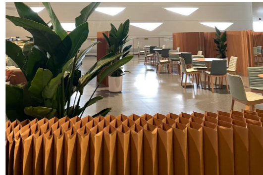
Coffee corner enclosure made of recyclable corrugated cardboard
