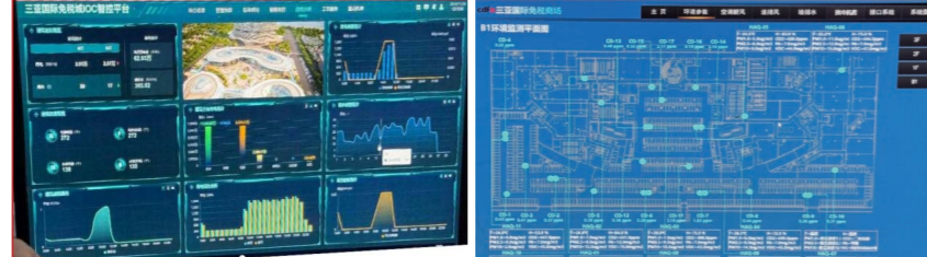
^ Automatic remote metering system, integrated energy management system, and air quality monitoring system (photo of Sanya International Duty-Free Shopping Complex Zone C)
