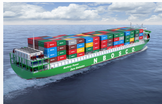
10,000-ton-class 740TEU Full Electric Container Vessel
